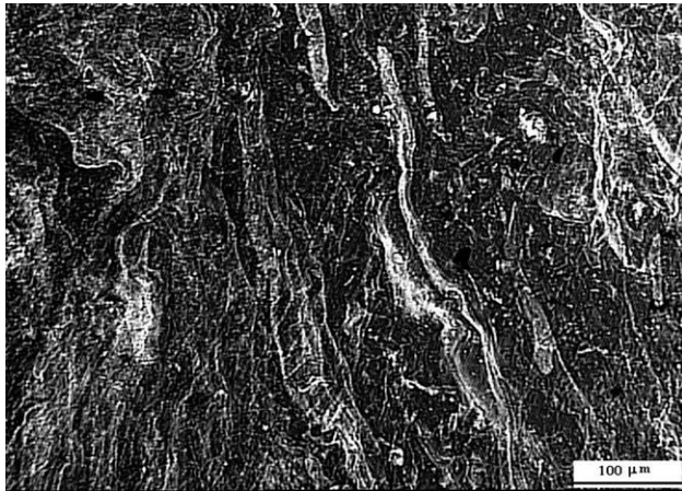
Figure 5 State of dispersion of 4% SBR in bitumen.
